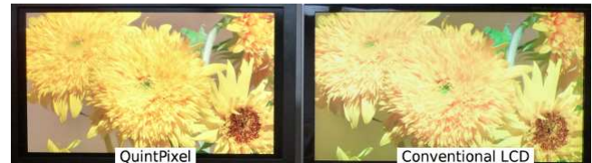
Figure 2: QuintPixel display (left) and its comparable conventional LCD (right). Note much deeper reproduction of yellow.
